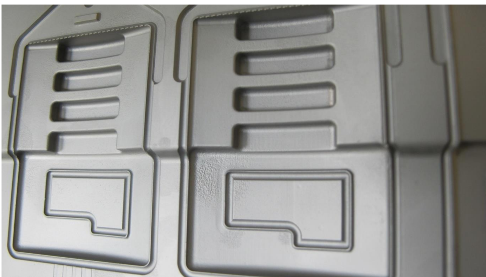
Figure 2. Detail of the repaired surface of the mould by DMX
